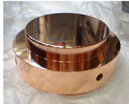
FIG. 1. Electrode used by the large electrode system for breakdown experiments. A pair of such electrodes facing each other symmetrically forms the interelectrode vacuum gap. The spacer separating the electrodes rests on the outer rim of the bottom electrode, and in turn supports the top electrode by the rim.
