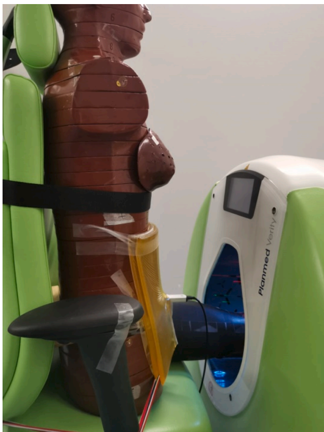
Fig. 3. Measurement setup with added bolus material for knee examination. For elbow examination bolus positioning was similar.
