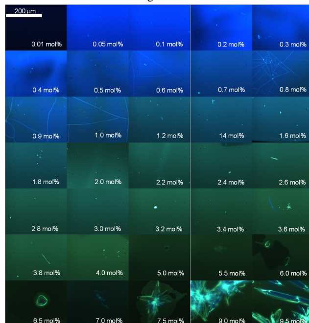
Figure 8. Fluorescence microscope images of PMMA films containing different BF 2 AVB concentrations.
