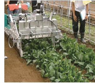
Fig. 17. State of harvesting by the automatic harvester
