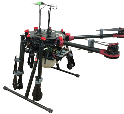
Fig. 2. The arms of Opt-copter can be folded which realize high portability. The light source is installed under the body.
