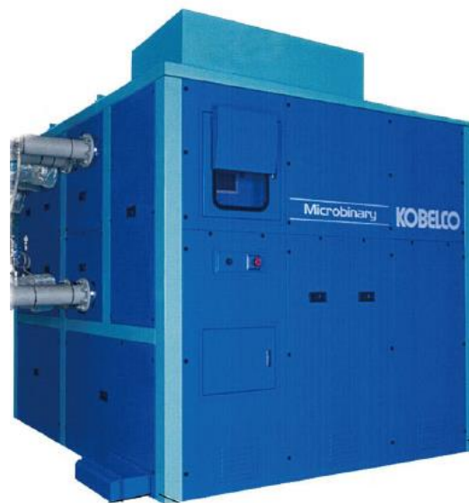
Figure 5-3 MB-70H ORC power generation from KOBELCO Company ( 60 kW e electrical capacities and using R-245fa as working fluid ) [24]
