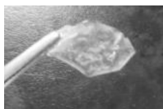
Fig. 8. A picture of after exposure of poly(2-MOM) film to conc. HCl aq vapor for 2 h.
