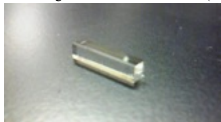
Figure 1 Lutetium Fine Silicate (LFS) is a newly developed inorganic scintillator with a size of 3 \times 3 \times 15 \text{ mm}^3
