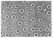
Figure 3. Phase Separation of PVA Film
