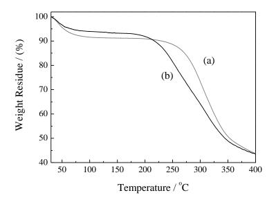
FIGURE 4. TG curves for SF fiber treated with 1.23 N  $I_2$ -KI solution for 168 h; (a) untreated SF, (b) iodinated SF.
