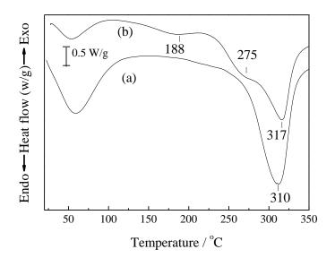
FIGURE 3. DSC thermograms of SF fiber treated with 1.23 N  $I_2$ -KI solution for 168 h; (a) untreated SF, (b) iodinated SF.
