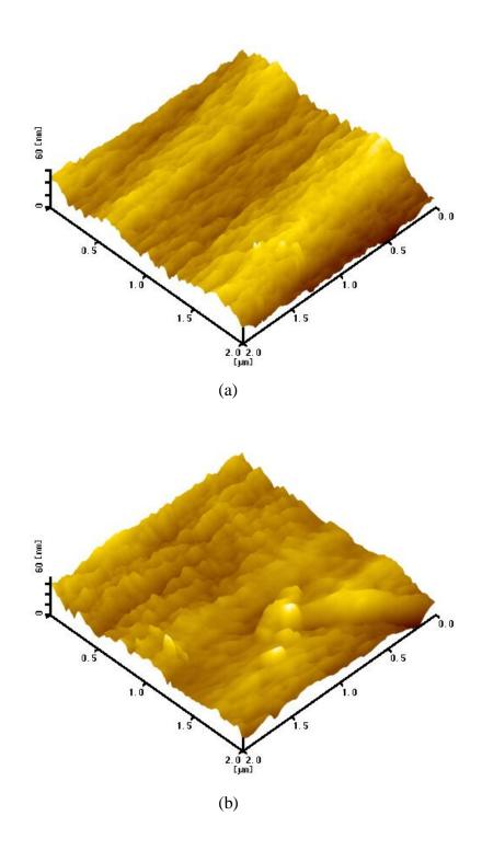
FIGURE 2. 3D AFM topographic images of SF fiber treated with 1.23 N  $I_2$ -KI aqueous solution for 168 h; (a) untreated SF, (b) iodinated SF.
