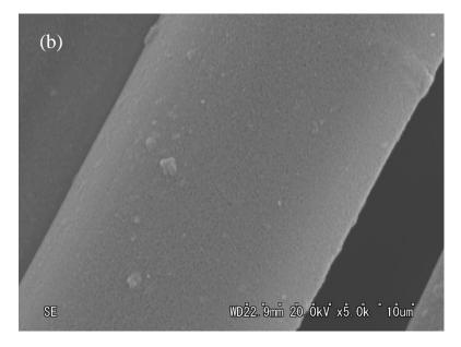
FIGURE 1. SEM images of SF fiber treated with 1.23 N  $I_2$ -KI aqueous solution for 168 h; (a) untreated SF, (b) iodinated SF.
