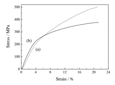
FIGURE 5. Stress-strain profiles of SF fiber treated with 1.23 N I<sub>2</sub>-KI solution for 168 h; (a) untreated SF, (b) iodinated SF.
