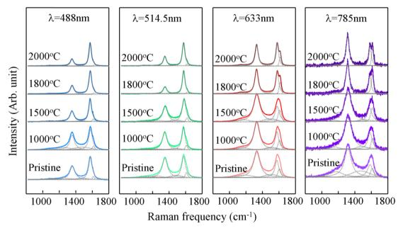
Fig. 4 Raman spectra of pristine N-doped MWNTs and thermally annealed N-doped MWNTs, in an argon atmosphere, at temperatures ranging between 1000 °C and 2000 °C, using four laser lines (488, 514.5, 633 and 785 nm).
