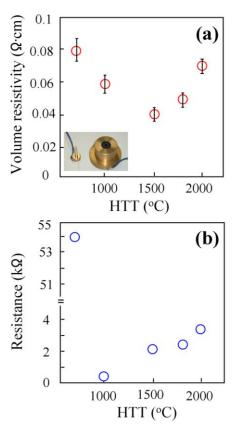
40 Fig. 2 (a) Variation in the volumetric resistivity of N-doped MWNTs as a function of heat treatment temperature at a density of 1.23 g/cm³; the inset shows the sample holder. (b) Variation of the electrical resistance of an individual N-doped MWNT as a function of heat treatment temperature.
