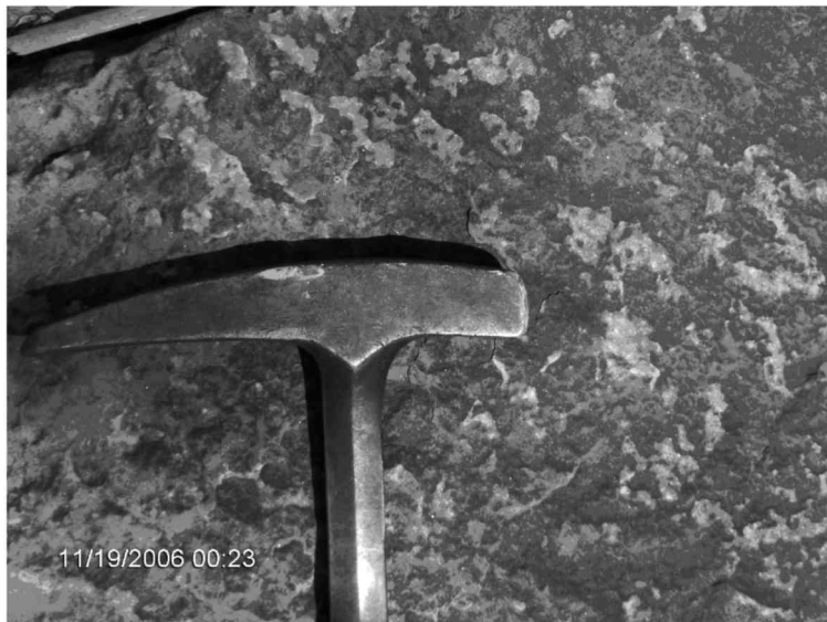
Fig. 25 : Slickenside observed on the fine grained sandstone on the right bank of the Tui Khola, about 500 m upstream from the confluence of the Tui Khola and Babai.
