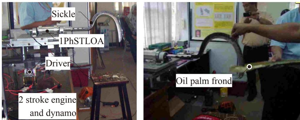
(a) Equipment setup for cutting evaluation.
