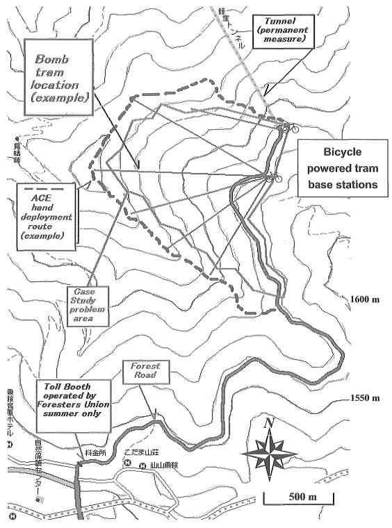
Figure 12 Azumi avalanche active control solutions map Example of a system of bomb trams strung from the Forest Road situated below and ACE hand deployment footpath (bombing route).
