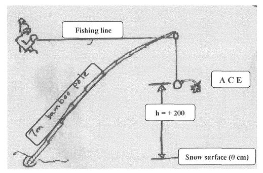
Figure 17 Improvised ACE aerial detonation technique
