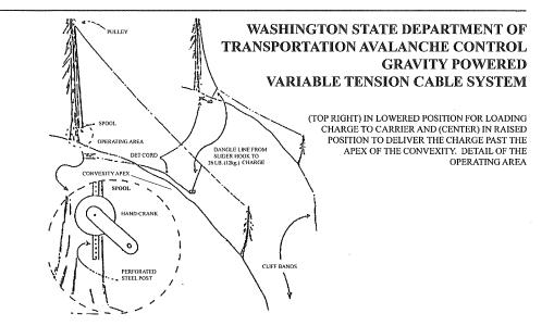
Figure 10 Lowering type bomb tram Image courtesy of Washington State Department of Transportation
