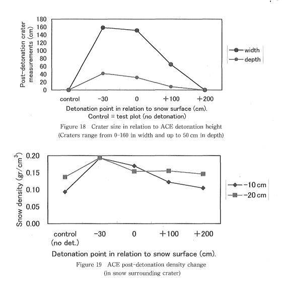
Mixed results were seen with charges deployed at heights of greater than  $\pm 100$  cm showing little evidence of explosion the snow surface in most snow types (Figure 18). Only when detonating at the surface or buried charges in soft snow conditions were depressions of a maximum width of  $\pm 150$  cm were created.
