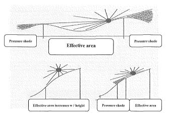
Figure 1 Explosion effective zone and shadow area Drawing based on original SLF document
