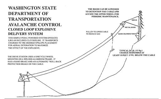
Figure 9 Raising type bomb tram Image courtesy of Washington State Department of Transportation
