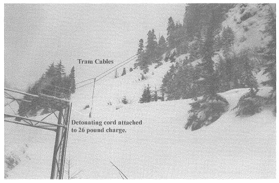
Figure 11 Bomb tram (raising type) shown with 12kg ANFO charge Photo courtesy of Washington State Department of Transportation Snoqualmie, Washington, USA
