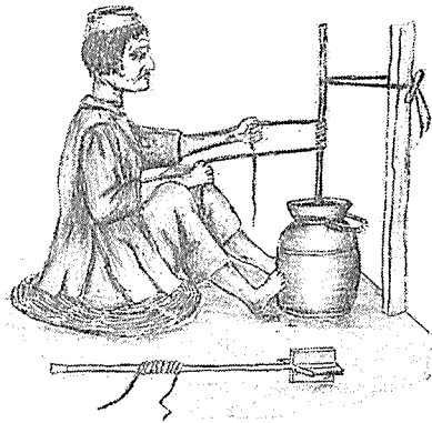
Fig. 4 Manufacture of butter with a rotary type churn (Thaykiy). (sketched by the authors).
