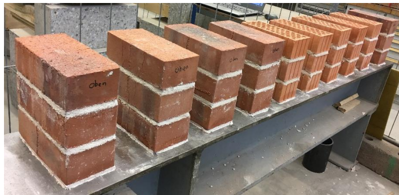
Fig. 4-8 Stack-bonded prisms for testing masonry compressive strength
