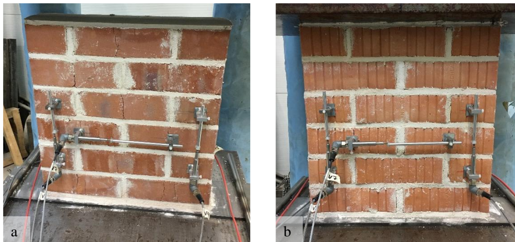
Fig. 4-7 Specimens according to EN 1052-1 (1998) for testing masonry compressive strength (a: solid clay brick masonry, b: perforated clay brick masonry)
