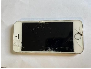
Figure 5.7- No.31 sample. The screen is surrounded by visible cracks.
