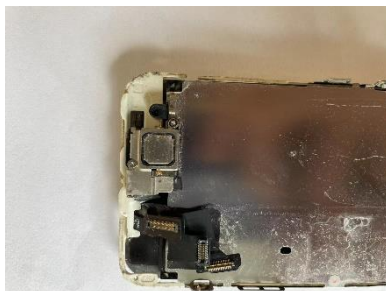
Figure 5.6- No.23 sample. The edges of the screen have obvious gaps and are seriously aged
