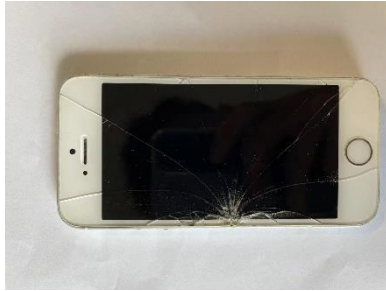
Figure 5.3- No.4 sample. One side of the screen is visibly cracked
