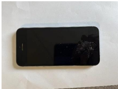
Figure 5.5- No.22 sample. The 'Home' key is off and the edge of the screen is cocked up
