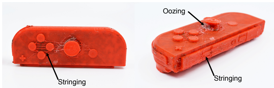
Figure 8.7: Fabricated case study product A with defects highlighted.
