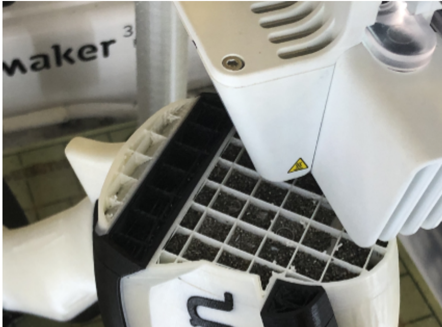
Figure 4.4: Design 3 being manufactured on an Ultimaker 3 Extended, with coarse iron filings and lead pellets contained within the infill.
