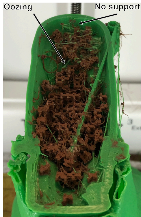
Figure 8.4: In-process issues with support structure deposition in case study B.
