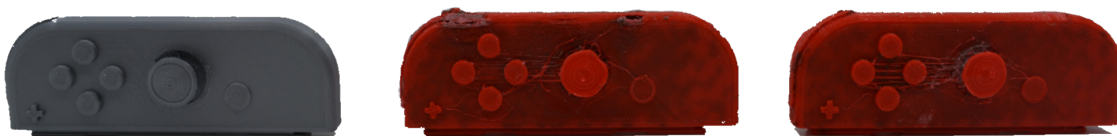
Figure 8.5: MEX fabrications of case study A with a conventional print (left), an initial fabrication with breakthrough from the interior and holes (center), and the final fabrication demonstrating a lack of retraction and oozing (right).
