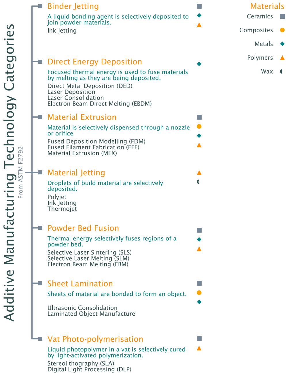
Figure 3.1: Additive technology categories, as specified by ASTM F2792 [22]. Adapted from information in “Overview on Additive Manufacturing” ([123, 138], with supporting information from [140]).
