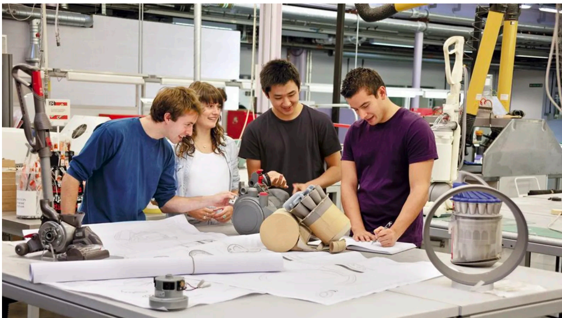
Figure 1.1: Dyson prototyping using sketches, cardboard, 3D prints and previous products as product prototypes (credit BBC [5]).
