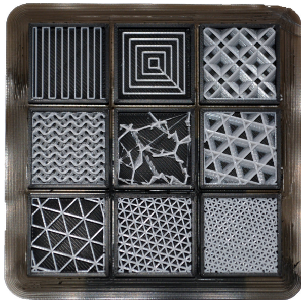
Figure 3.2: Different infill designs that can be printed. From left-right, top-to-bottom: Lines (0 degrees), concentric, octet, gyroid, lightning, cubic, triangles (20%), triangles (50%) and triangles (80%). Printed using an Ultimaker S3, sliced using Cura 4.12.1.
