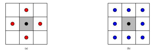
Figure 6.3: (a) Compact face-based stencil on the example of a structured quadrilateral mesh. (b) Extended node-based stencil on the example of a quadrilateral triangular mesh.
