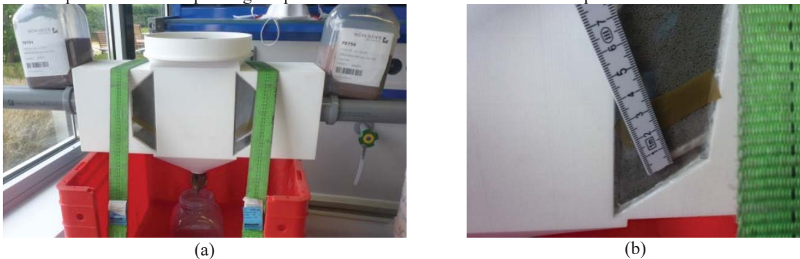
FIGURE 11. Pretesting of 3-D printed plastic compensator a) compensator in operation, b) deflection measurement
