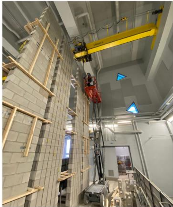
Figure B.16: Placement of NSM reinforcement using overhead crane
