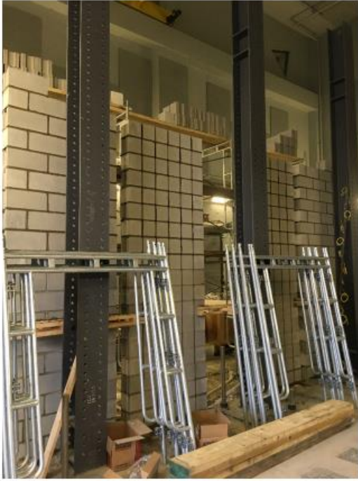
Figure B.5: Second stage of slender wall construction
