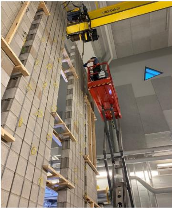
Figure B.16: Placement of NSM reinforcement using overhead crane
