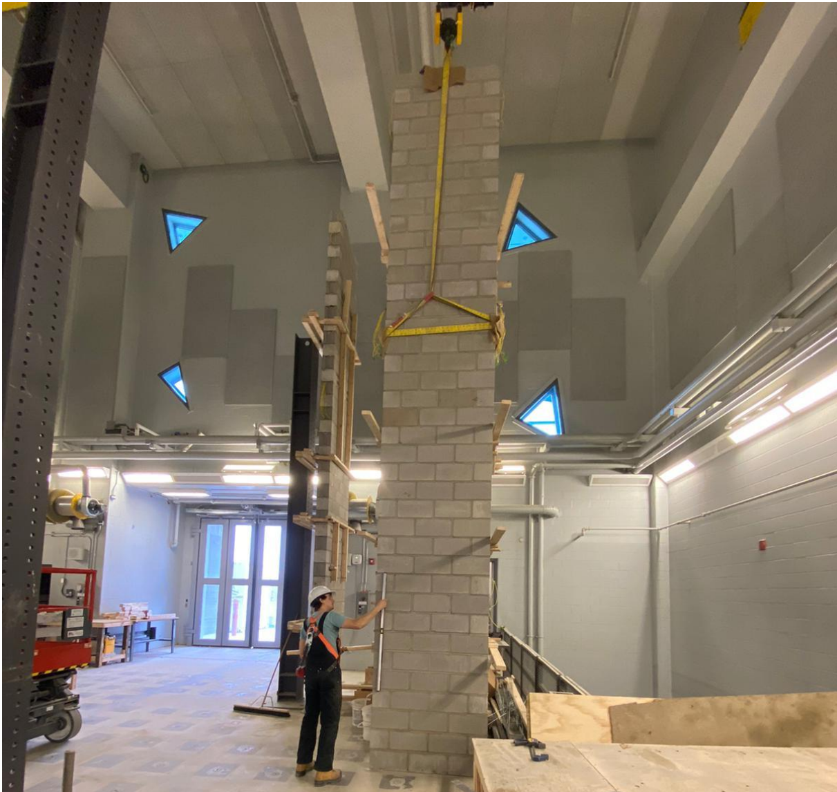
Figure B.17: Lifting of slender reinforced masonry wall
