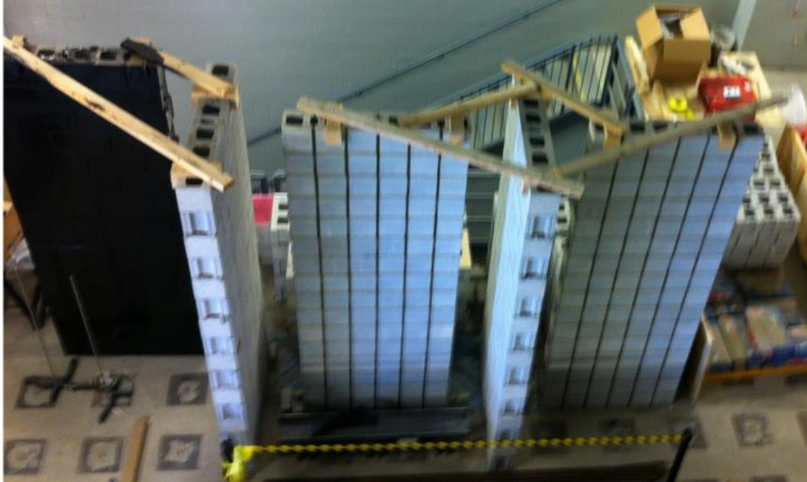
Figure A.9: Completed walls braced against each-other for stability
