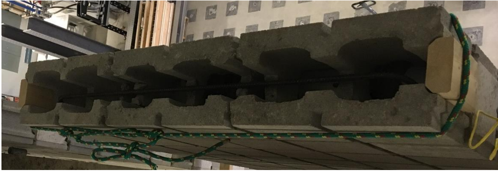
Figure B.15: Reinforcement and flashing for grouting of top course of masonry: SRCMU wall
