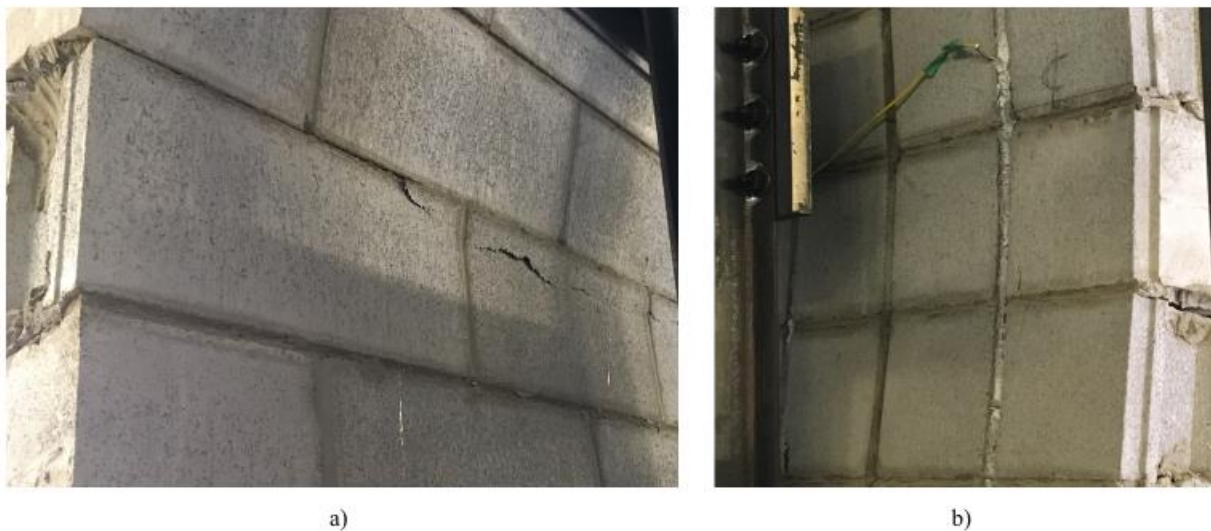
Figure 4.19: Compression and rotation of mortar joints at the ultimate displacement: a) CG3200, and b) NG3200
