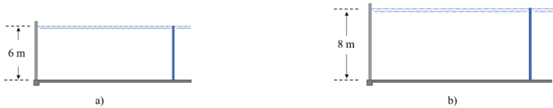
Figure D.2: Typical elevation of warehouse wall: a) small warehouse, and b) large warehouse
