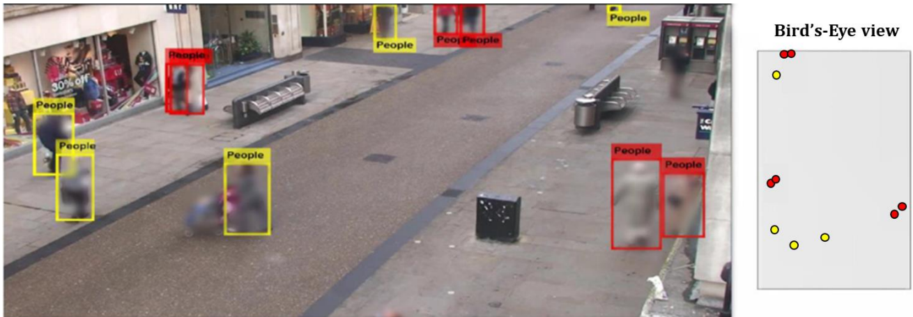
Figure 1-3: Real time monitoring system for physical distancing detection (Meivel et al., 2021)
