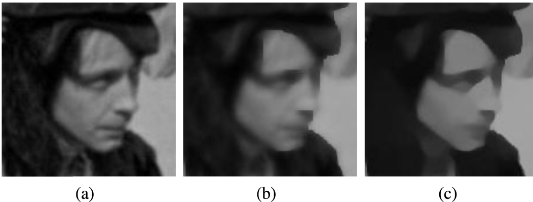
Figure 2.2: An example from [4] that compares GLR and GTV priors in image deblurring problem. (a) Image blurred by Gaussian blur. (b) Image filtered with SDGLR. (c) Image filtered with RGTv.
