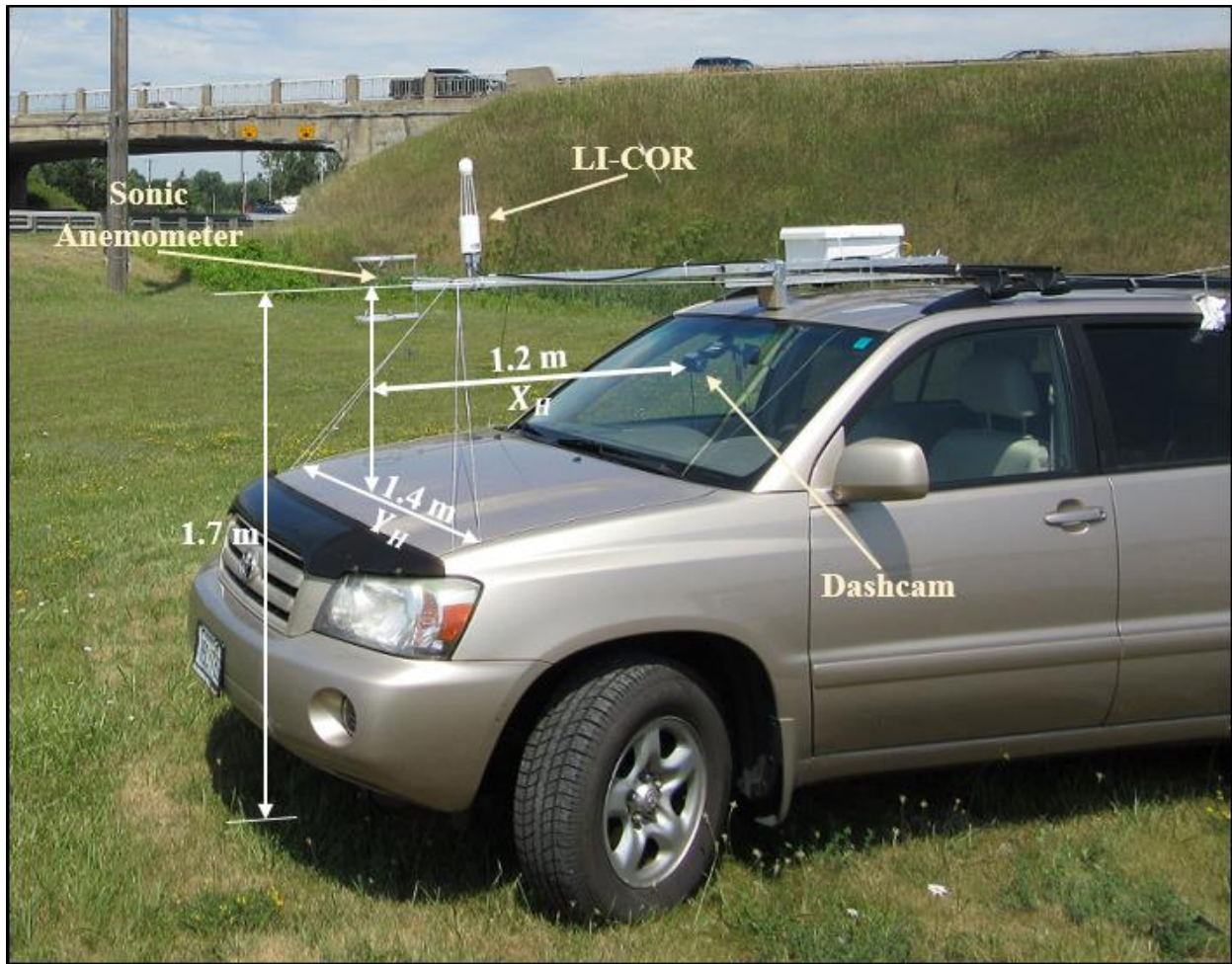
Figure 2.3: The mobile laboratory developed at York University. Shown are the location of the sonic anemometer, the LI-COR gas analyzer and the dashcam. Physical measurements are superimposed.
