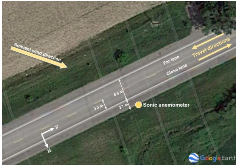
Figure 5.2: A schematic showing the location of the sonic anemometer and the estimated distances of the highway (estimated from Google Earth). The coordinate system of the sonic anemometer used in this investigation is given in the image (the vertical velocity component is upward, but it is not shown in the figure), as well as the vehicle travel directions.
