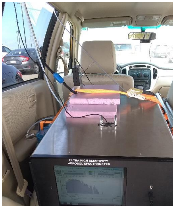
Figure 4.1: The aerosol sampling setup used during the 2019 study. A view of the inside of the instrumented car is shown.
