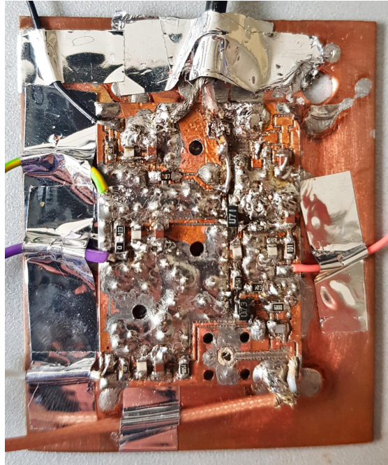
Figure 5.2: The assembled cryogenic amplifier. Starting from right side with the pink cable the cables are in clockwise order: Drain Stage1, Output, Drain Stage2, Gate2 Stage1, GND, Gate1 Stage1, Input
