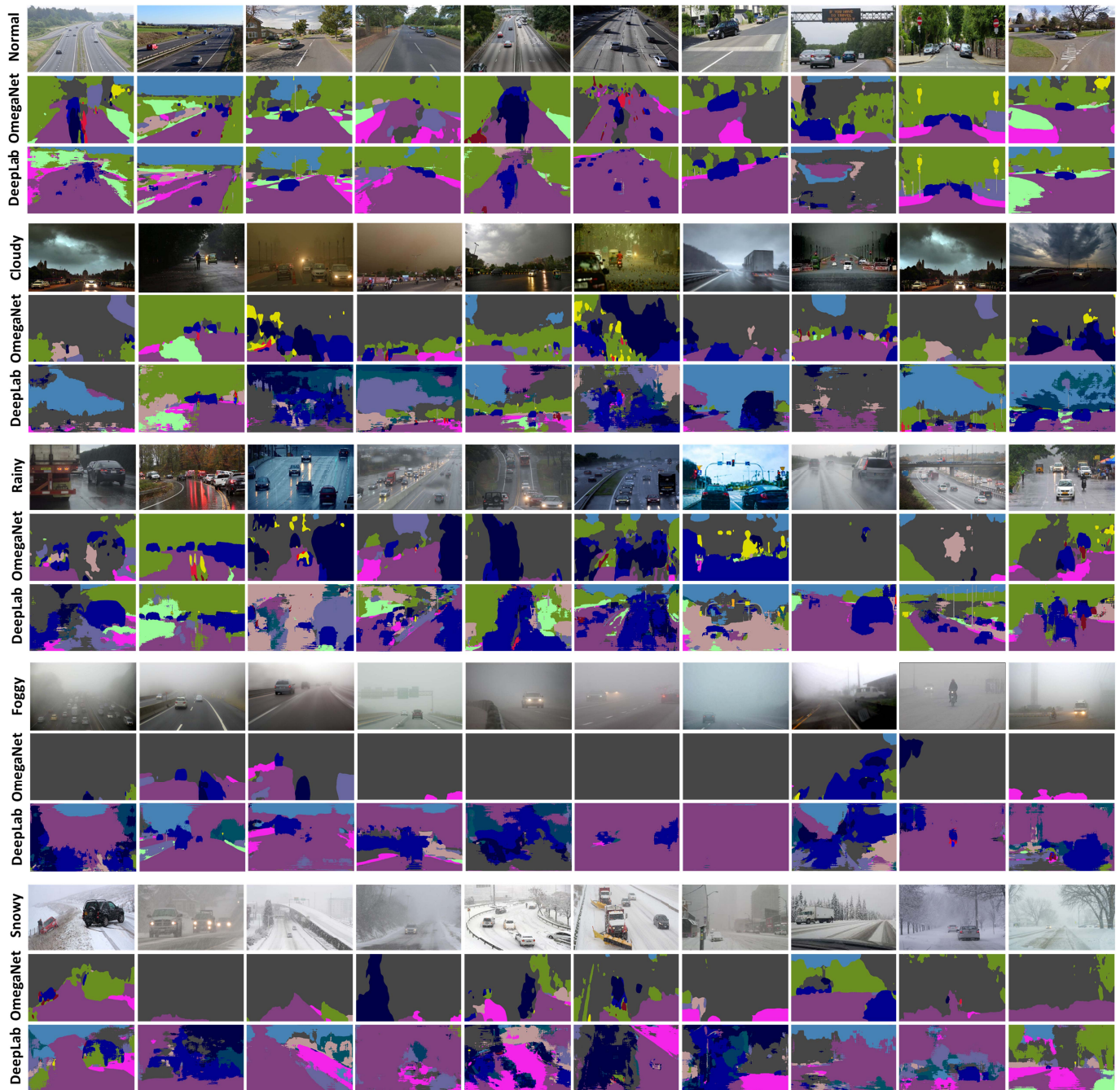
Fig. 5. Visual segmentation results of various deep segmentation models over input images having variable weather conditions such as snow and fog. The segmented maps of DeepLab and OmegaNet are not trustworthy for an autonomous vehicle’s scene understanding.
