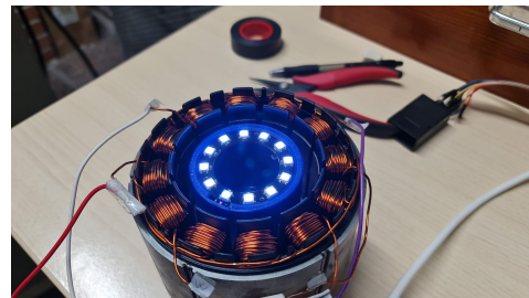
(b) Testing mount with motor mounted
