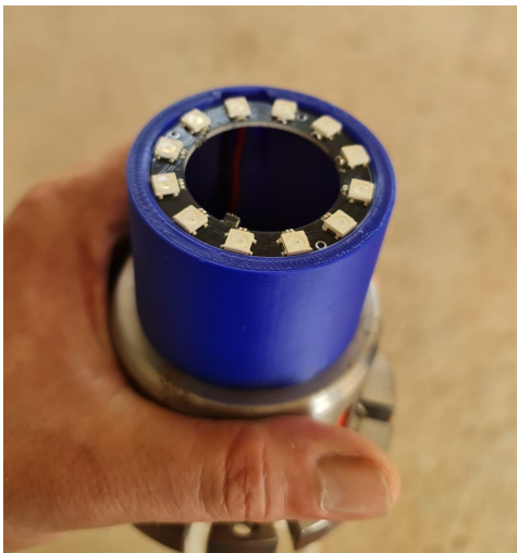
(a) Testing mount with LED ring assembled on top
