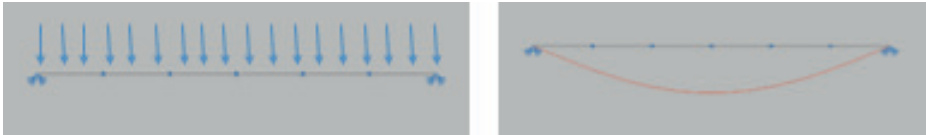
Figure 6. Beam subjected to uniform applied load and its corresponding Bending Moments Diagram.
