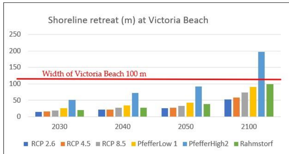
Figure 6. Shoreline retreat (m) at Victoria Beach projected for the years 2030, 2040, 2050, and 2100, according to the different models and scenarios.
