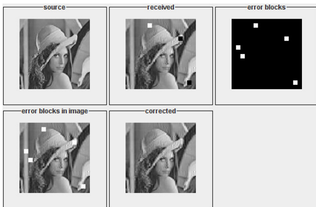
Fig. 7 IAC-WNTMAC at SNR 2.5 with Turbo Codes of rate-1/3
