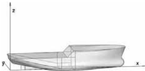
Figure 1. Reference system for the hydrostatics calculation.
