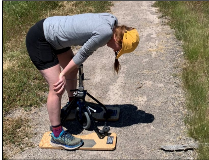
Figure 3.5: Testing with the Beneficial Designs rotational penetrometer.
