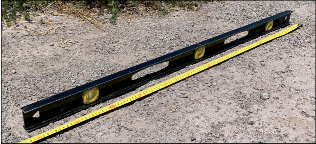
Figure 7.1: Roughness profile measurement setup: vertical distances between the level and the ground were measured at 10 cm increments.
