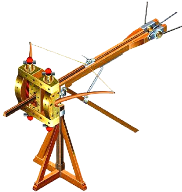
Fig. 1. Author's virtual reconstruction of a Roman catapult with torsion motor.
