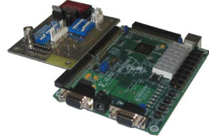
Fig. 7. FPGA based power-factor controller: (a) block diagram and (b) prototype controller.
