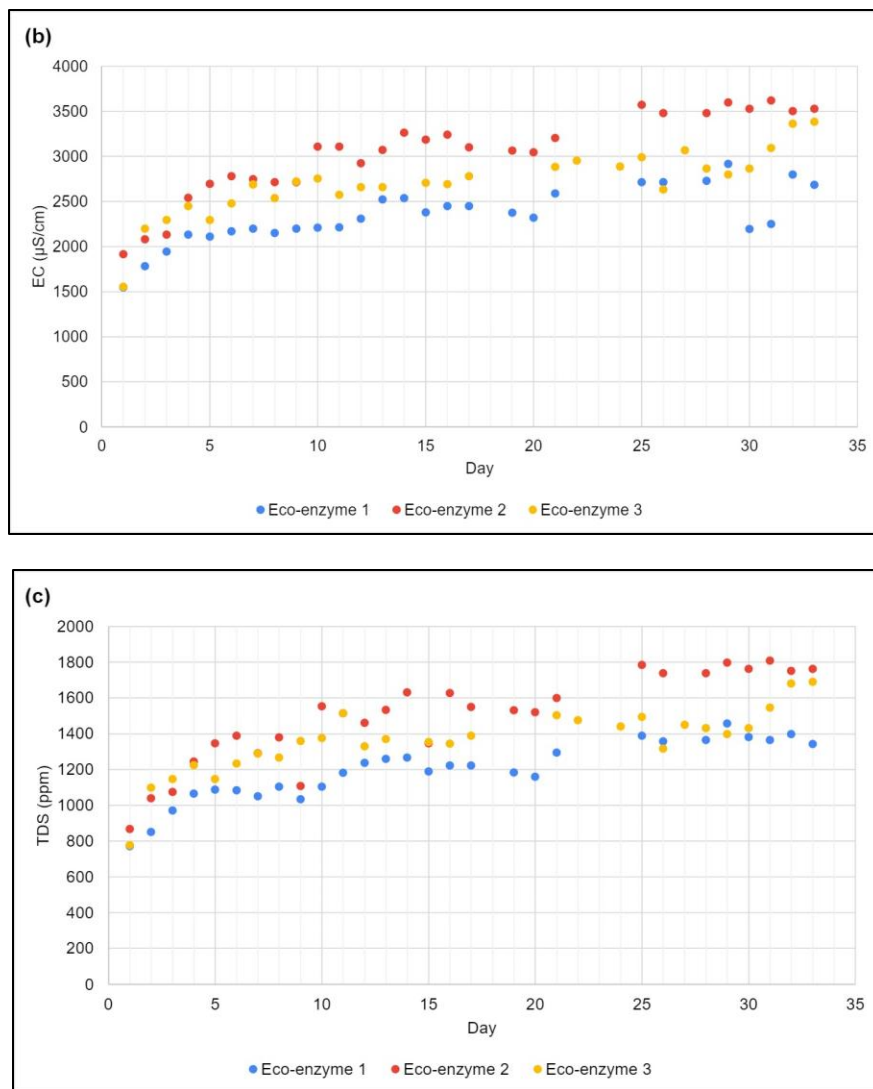
Figure 1. Changes in (a) acidity (pH), (b) Electric Conductivity (EC), and (c) Total Dissolved Solid (TDS) for three eco-enzyme products from day 1 until day 33. The green dot shows the pH measurement results for the eco-enzyme 1, the blue point shows the pH measurement result for the eco-enzyme 2, and the yellow point shows the pH measurement result for the eco-enzyme 3.
