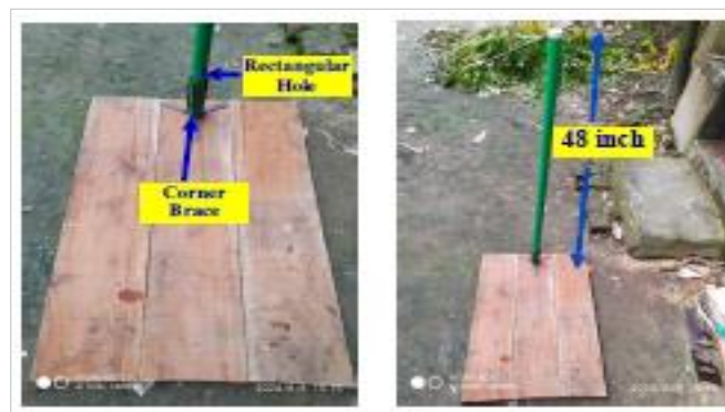
Figure 7: Attachment of pipe with the wooden base
