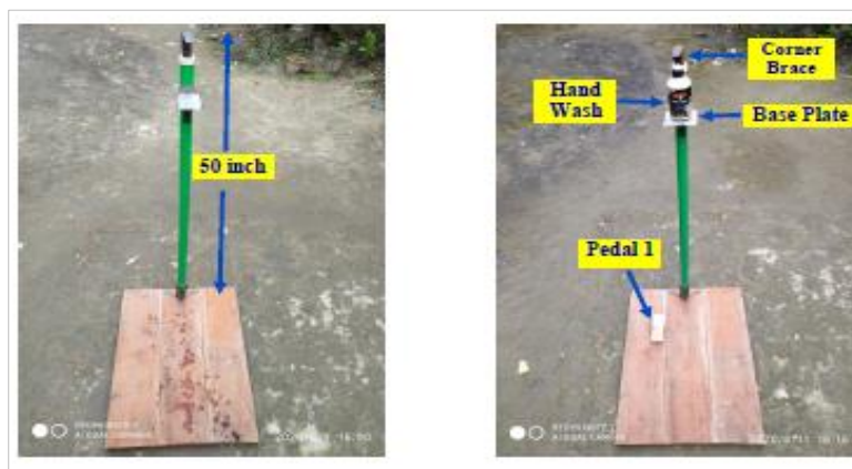
Figure 8: Attachment of Corner Brace and Pedal
