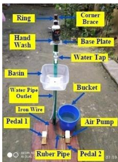
Figure 10: Final setting of the "Foot Press Hand Washing Device"
