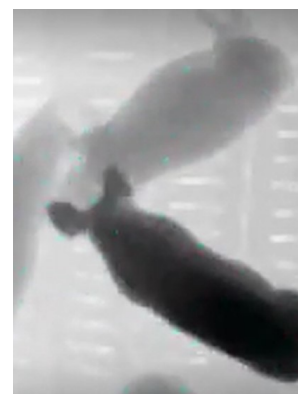
Left: RFID ear tagged pigs; Right: Greyscale 3D camera image—standing pigs are closer to the camera so appear darker than lying pigs
