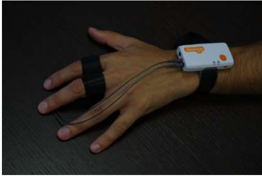
Figure 5: Shimmer3 GSR for the Capture of Galvanic Response Signals from the Skin, Located in the Proximal Phalanx of the Left Hand.
