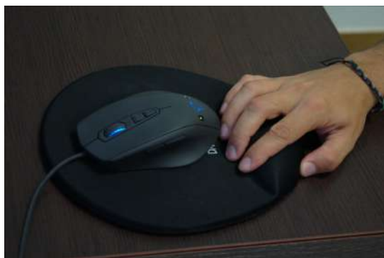
Figure 6: Mionix Naos QG Mouse for the Capture of Galvanic Response Signals from the Skin Located in the Right Hand.
