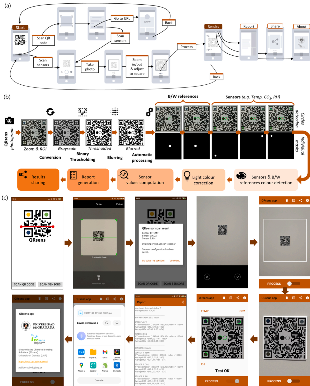
Fig. 3. (a) Application user flow showing the path that the user follows through the developed smartphone app interface to complete the acquisition of the QRsens device. (b) Flow diagram describing the image processing sequence conducted by the smartphone application. (c) Screen captures of the smartphone application corresponding to different steps of the described user flow.
