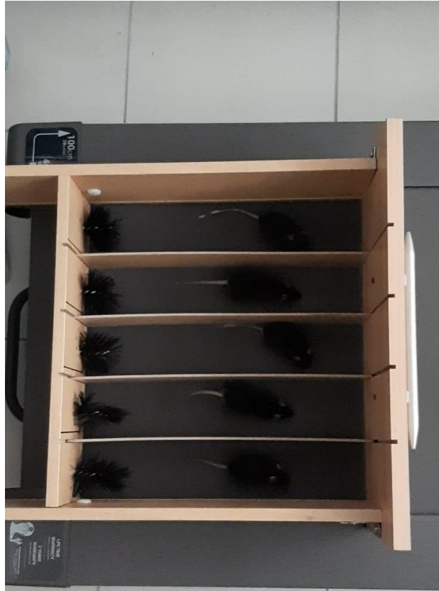
Figure 9. Treadmill test with separate lanes for each animal.
