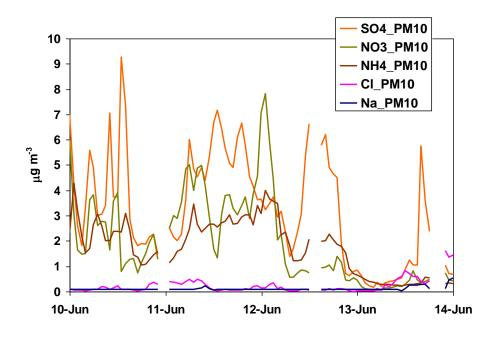
Figure 17: Concentrations of particulate matter (PM<sub>10</sub>) sampled by the MARGA between 10 and 14 June 2007
