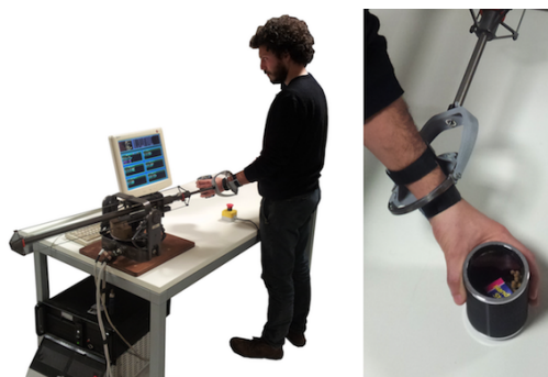
Fig. 1. Overall system employed for the generation of tremor composed by a haptic interface, controller and a novel end-effector spherical wrist.
