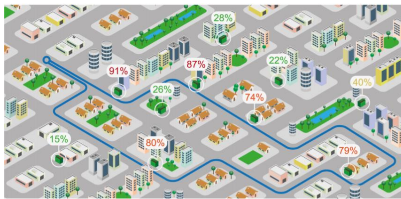
Figure 6- Current solution of the waste management system, with route optimization based on capacity available [28].
