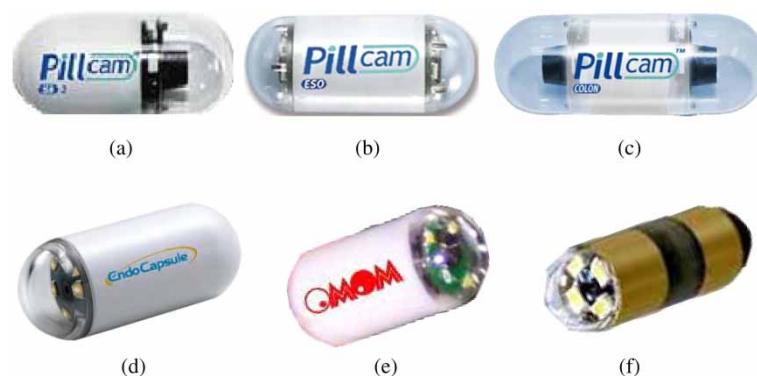
Fig. 1 Current commercially available swallowable camera capsules include (a) PillCam SB2, (b) PillCam ESO, (c) PillCam Colon, all by Given Imaging, Inc., as well as (d) EndoCapsule of Olympus, Inc., (e) OMOM of Jinshan Science and Technology Group, and (f) MiRo of Intromedic Co. These capsules carry cameras into the GI tract for visual inspection. While most of the capsules shown are designed for the small intestine, PillCam ESO is an oesophageal capsule and the PillCam Colon carries two onboard cameras for use in the large intestine. All capsules are 11 mm in diameter \times 26 mm in length except for OMOM (13 mm \times 27.9 mm), MiRo (10.8 mm \times 24 mm) [14], and PillCam Colon (11 mm \times 31 mm) [15]
