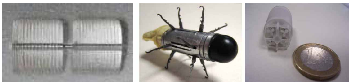
Fig. 7 Photos of various capsules that utilize internal locomotion: (left) an earthworm-like capsule that uses SMA actuation for extension and contraction (©2005 IEEE) [65], (centre) the 12-legged capsule developed by Valdastrì et al. [10, 75], (right) a propeller-driven capsule that acts like a miniature submarine in the stomach [21]
