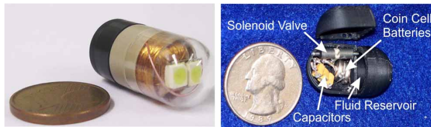
Fig. 12 (Left) Prototype capsule developed by Lenaerts et al. (©2007 Elsevier) [102], which is capable of transmitting 150 mW through inductive coupling. (Right) The prototype fluid-powered capsule of Toennies and Webster [88]
