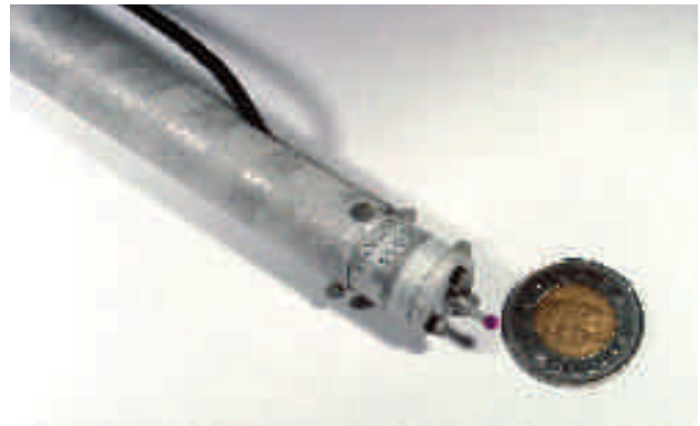
Figure 1. The sensor used to acquire force and torque information, alongside a coin to indicate scale.
