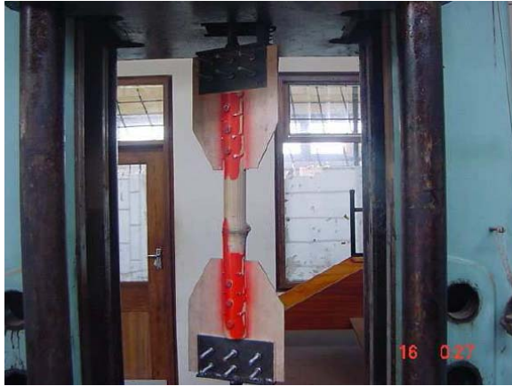
Fig. 13: mechanical test on single joint
