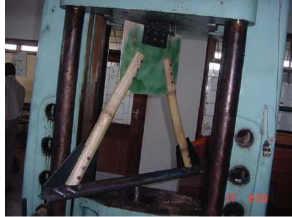
Fig. 14: mechanical test on double joint
