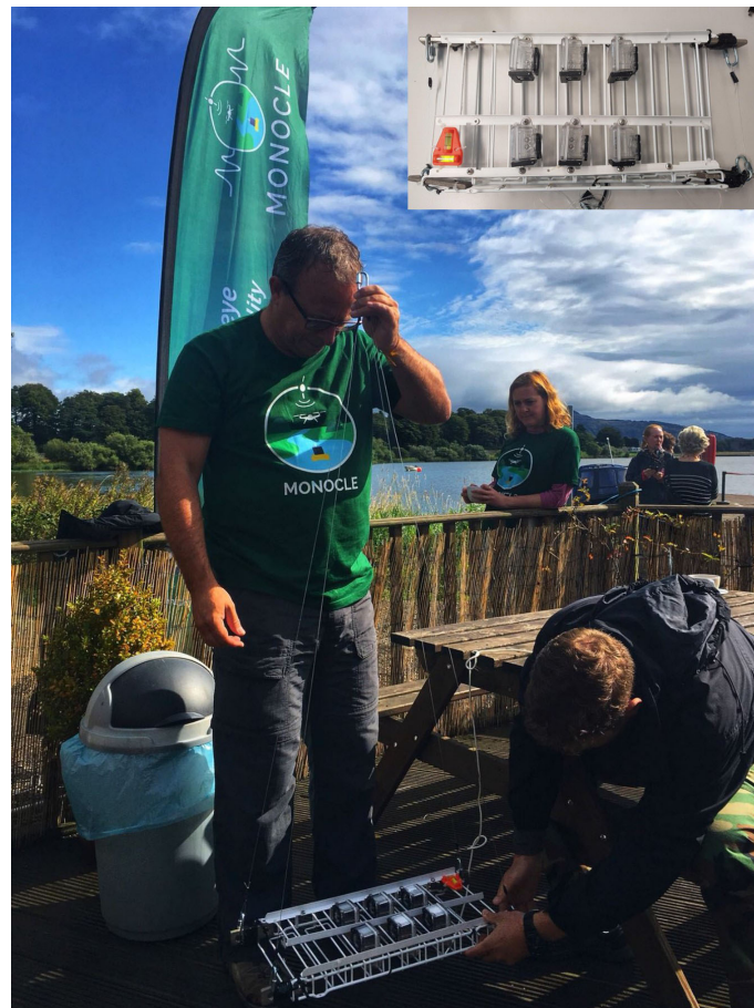
FIGURE 3 Concurrent measurements to derive theoretical K_d uncertainty. The in situ measurements took place in the Stirling's University campus (Airthrey Loch) and in the Loch Leven, in August of 2018. Six KduPRO (numbered as 13, 14, 15, 17, 18 and 19) were placed in the same plane at 1 m depth, doing measurements for 15 minutes at noon.
