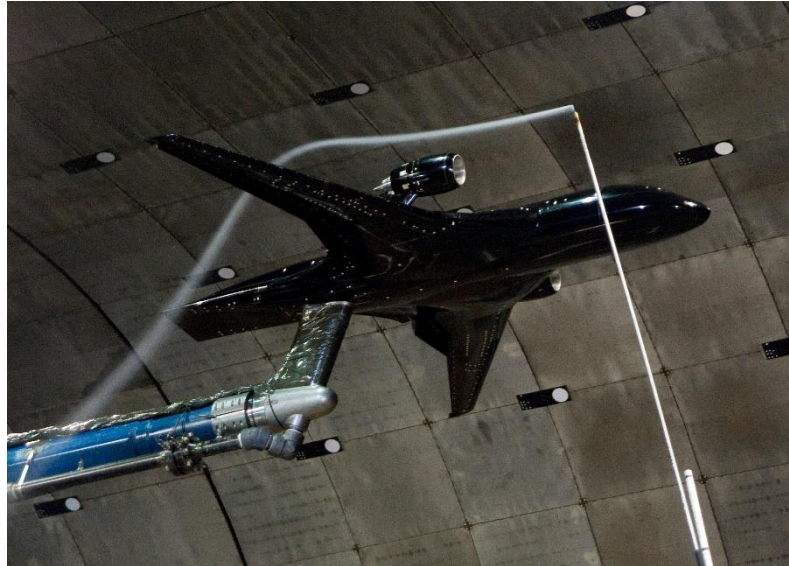
Figure 15. AMELIA model in the NASA Ames 40'x80' wind tunnel with smoke flow visualization showing the streamline turning from the active circulation control. (NASA.gov)
