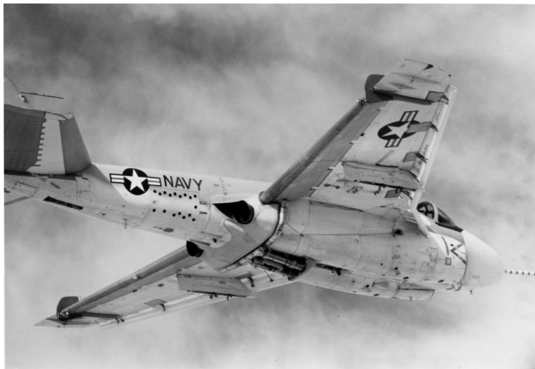
Figure 10. Modified Navy/Grumman A-6A aircraft with circulation control being tested in 1977 [17]
