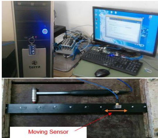
Fig 1 – Experimental set-up for vibration CFRP beam
