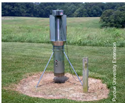
Fig. 6.11. A commercially manufactured blacklight trap for capturing nocturnal insects like VLB.
