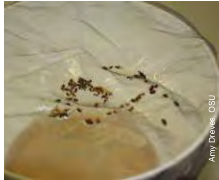
Fig. 3.29. Plastic wrap with holes used to separate SWD specimens from trap bait.
