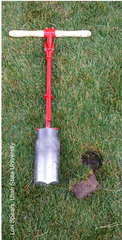
Fig. 7.20. Soil corer used to collect soil and root samples when JB damage to turf is suspected.
